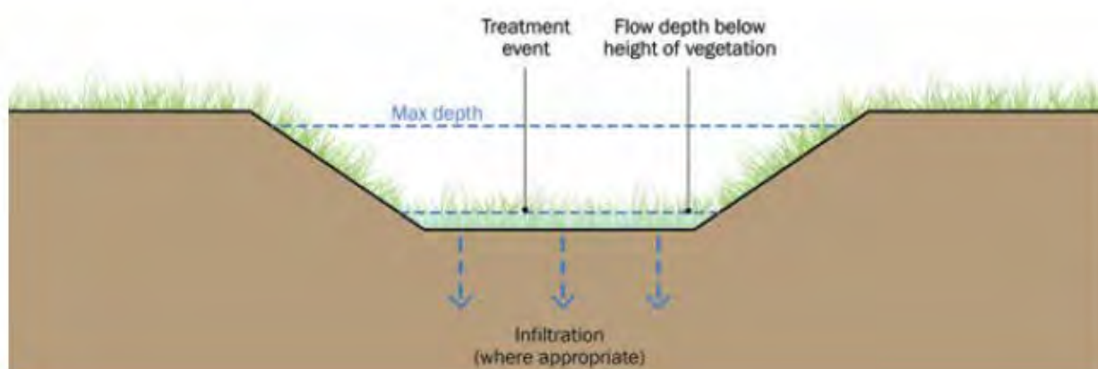
Figure 7-3 Swale: Conceptual Design Details
